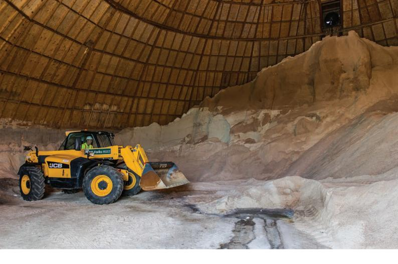
processed on site from inert construction and demolition waste, imported from other projects in the south east of England.. This represents 92% recycled content for bulk materials and a saving of 35,000 tonnes of embodied carbon. Where use of primary aggregate was unavoidable, responsible procurement was undertaken in line with BES 6001.
